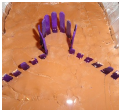
V-weir showing difference in post heights
