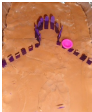
V-Weir, fish swims over barrier at high tide
